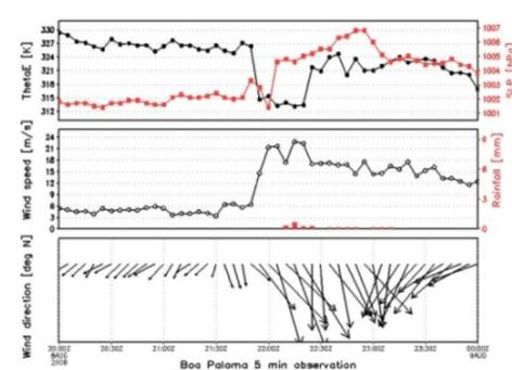
Fig. 3 Time series of the Boa Paloma meteorological station measurements every 5 minutes. The upper pictures show time series of  $\theta_{eA}$  in black (unit of measure in K, left axis), surface level pressure in red (unit of measure in hPa, right axis). The center picture shows time series of wind velocity (unit of measure,  $\text{ms}^{-1}$ ). The lower picture shows the time series of wind direction and intensity in vectors.
