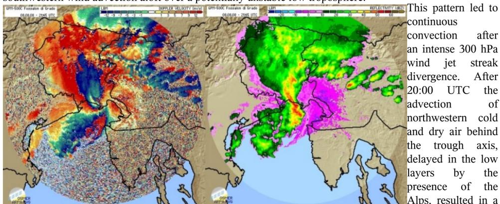
Fig. 2 LBM (Lowest Beam Map) reflectivity -left- and Doppler velocity -right- signatures from OSMER Fossalon radar at 21:45 UTC. Please note that the Doppler signature is affected by multiple folding.
