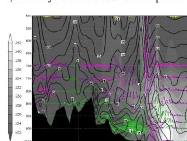
Fig. 6 WRF model cross section along density current direction (north-south). Shaded grey is  $\theta_{eA}$  (scale in K on the left); isochants in black contours ( $\text{ms}^{-1}$ ), green vectors are exiting winds (horizontal westward component), violet vectors are sheet-parallel winds. Black shapes at the bottom are Alps.
