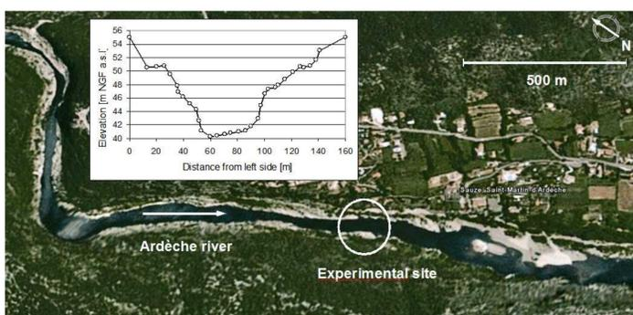
Aerial view (Google Earth) of the Ardèche river at Sauze-St Martin, and cross-sectional profile used for LSPIV discharge computation.
