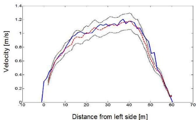
Comparison of depth-averaged velocities obtained with ADCP and LSPIV
