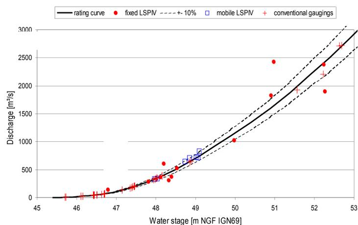
Comparison of mobile/fixed LSPIV discharge measurements with the rating curve and conventional gaugings (ADCP/current meter)
