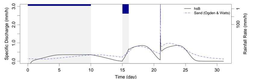
Fig. 5. Comparison of the hsB and 3-D coupled surface-subsurface models on a non-convergent hillslope (with a zero-flow condition applied at the downstream boundary).
