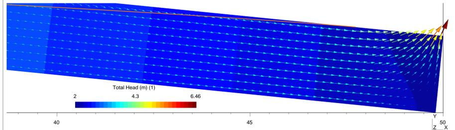
Fig. 4. Total pressure head network and fluxes in the hillslope after 10h, i.e. a 300 mm rainfall amount (with a zero-flow condition applied at the downstream boundary).
