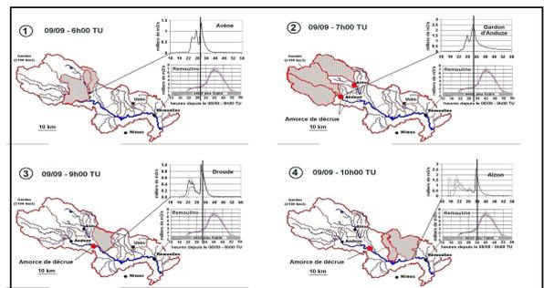
Figure 4: Reconstruction of the time sequence of the 2002 Gard river flood, the tributaries where the peak discharge occurs appear in grey
