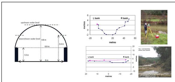
Figure 1: Example of surveyed river cross-sections (blue) and high-water marks (purple) after the 2002 Gard floods
