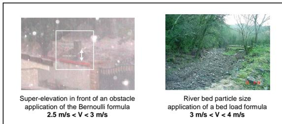
Figure 2: Illustration of clues used to evaluate flow velocities
